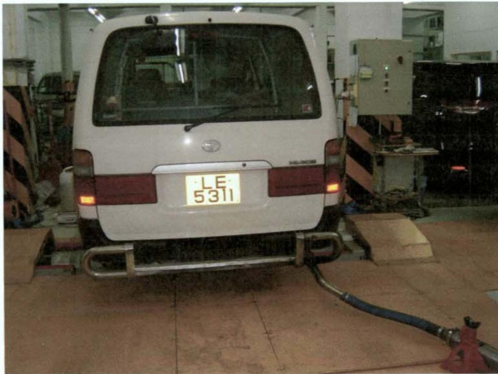
Photo 1. (Urban Cruise Simulation Test on Chassis Dynamometer)
