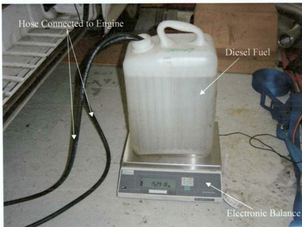
Photo 2. (Measure Fuel Consumption)
